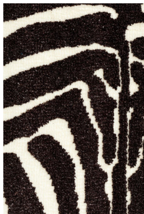
Figure 2: Sample tufted on Colortec with a combination of standard acrylic yarn (white) and fancy polyester (black)
