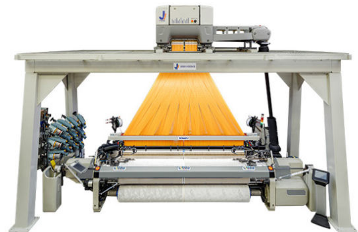
Figure 3: Ji jacquard with 2.688 hooks on top of a rapier loom weaving designs on double width in 8 repeats
