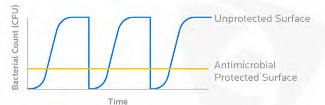
Blue Line - periodic disinfection of an untreated surface Orange Line - effect of a treated surface preventing organism growth
