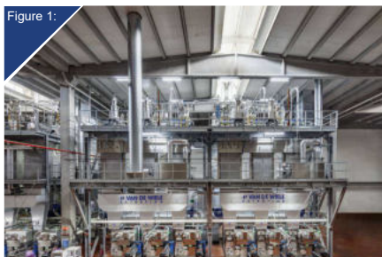
Figure 1: A tricolor BXE extrusion line running in a carpet weaving mill in Turkey
