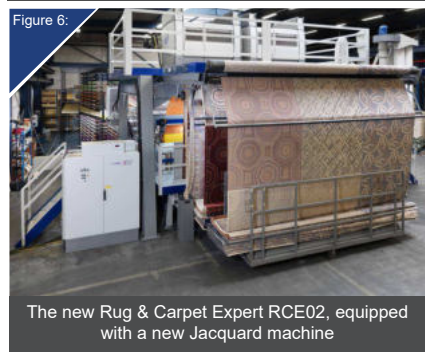
Figure 6: The new Rug & Carpet Expert RCE02, equipped with a new Jacquard machine
