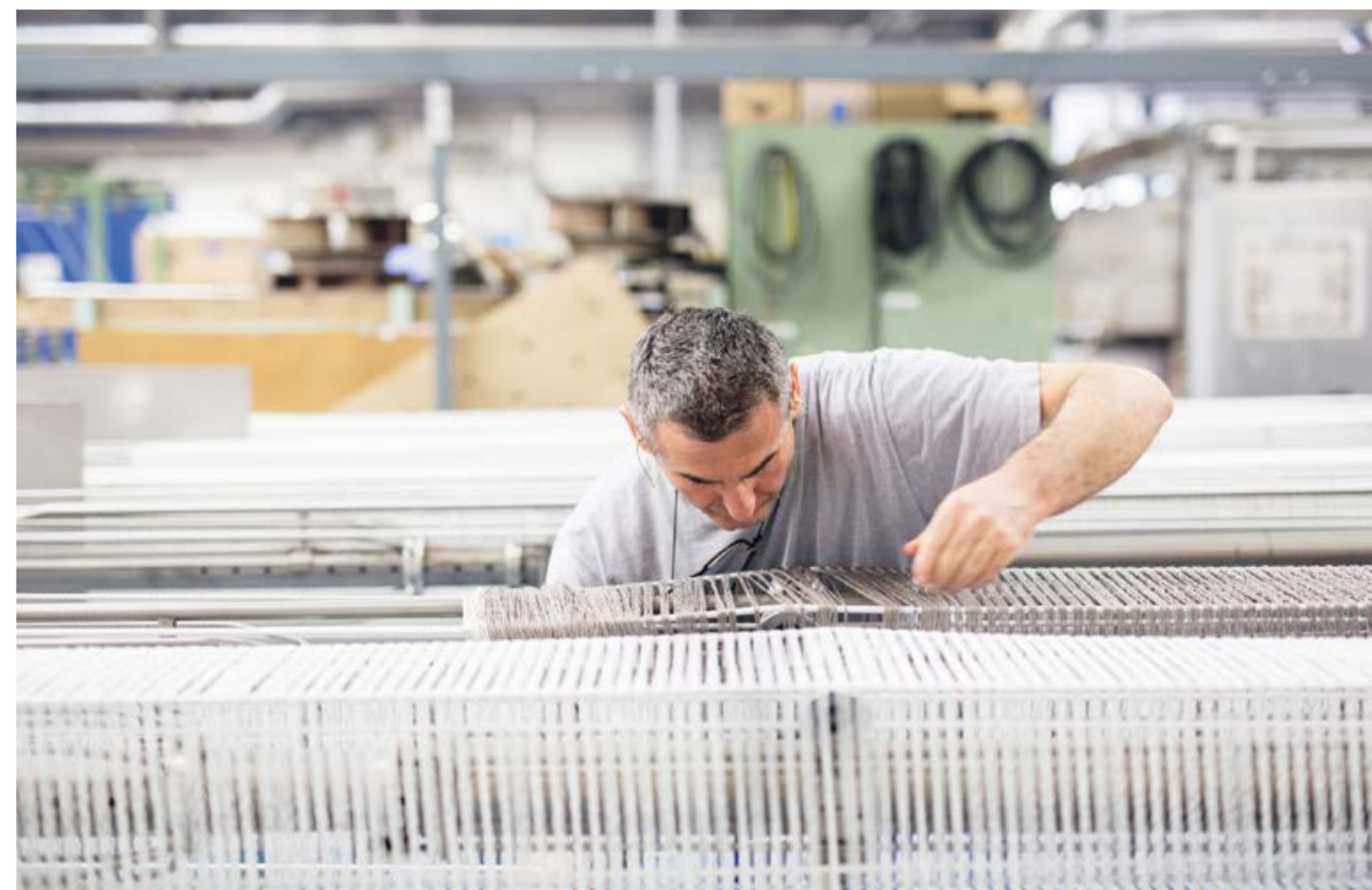
Because most carpet isn't designed to be recycled, Aquafil developed the custom machinery this worker is operating, to separate the waste material into three main ingredients. Photography: metropolismag
