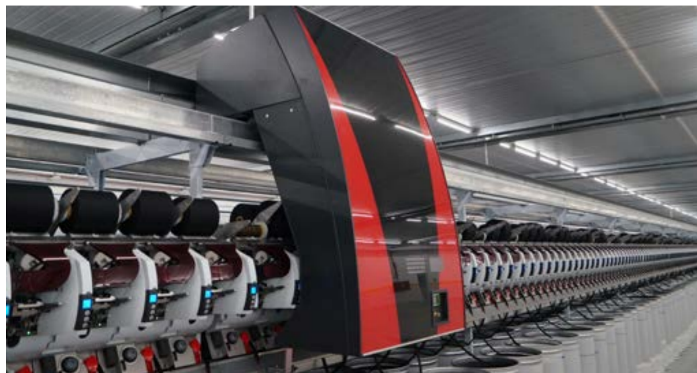
Autocoro 11 rotor-spinning machine for producing yarns from recycled fibres.
