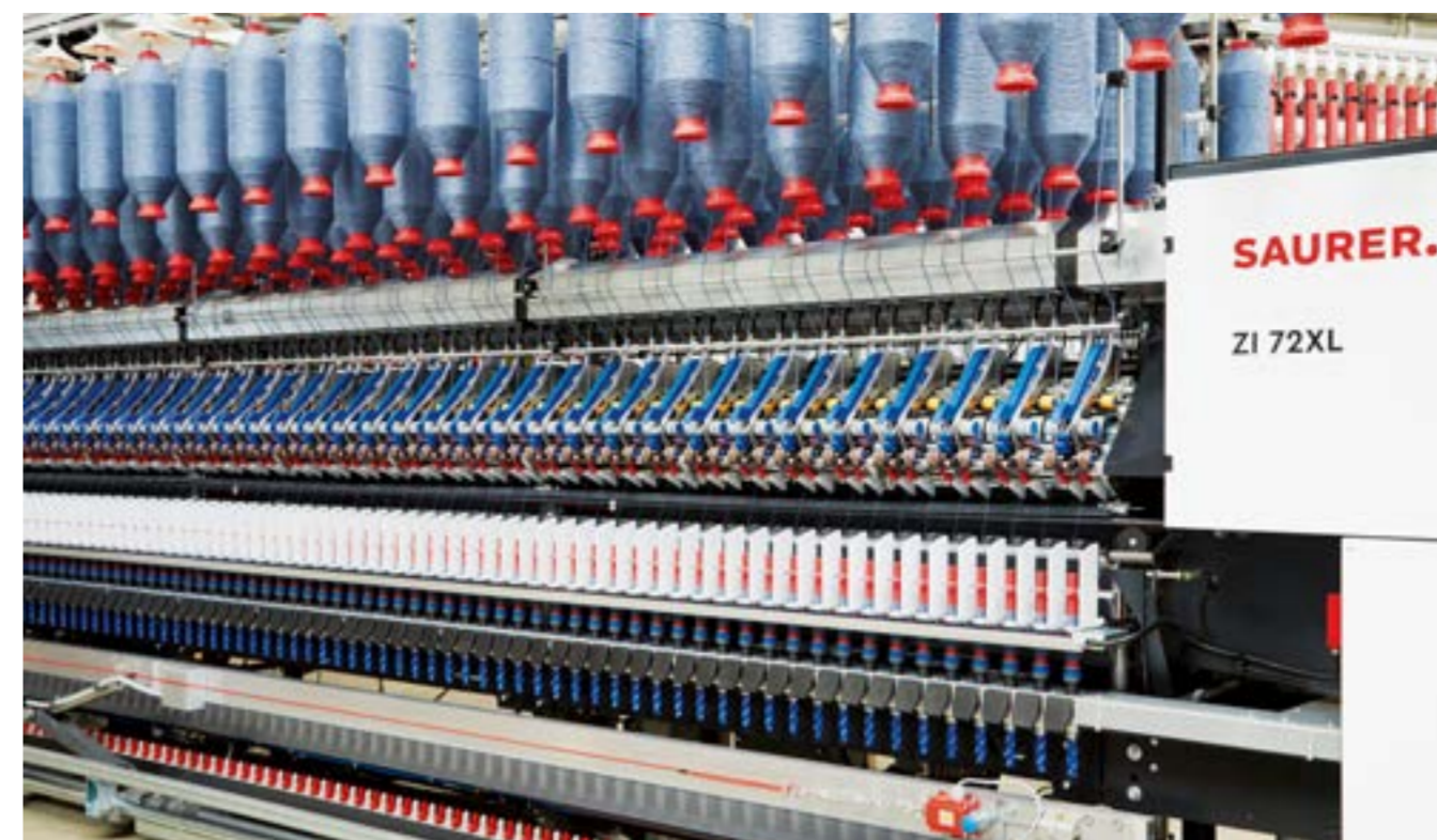
ZI 72XL compact-spinning machine processes recycled yarn.
