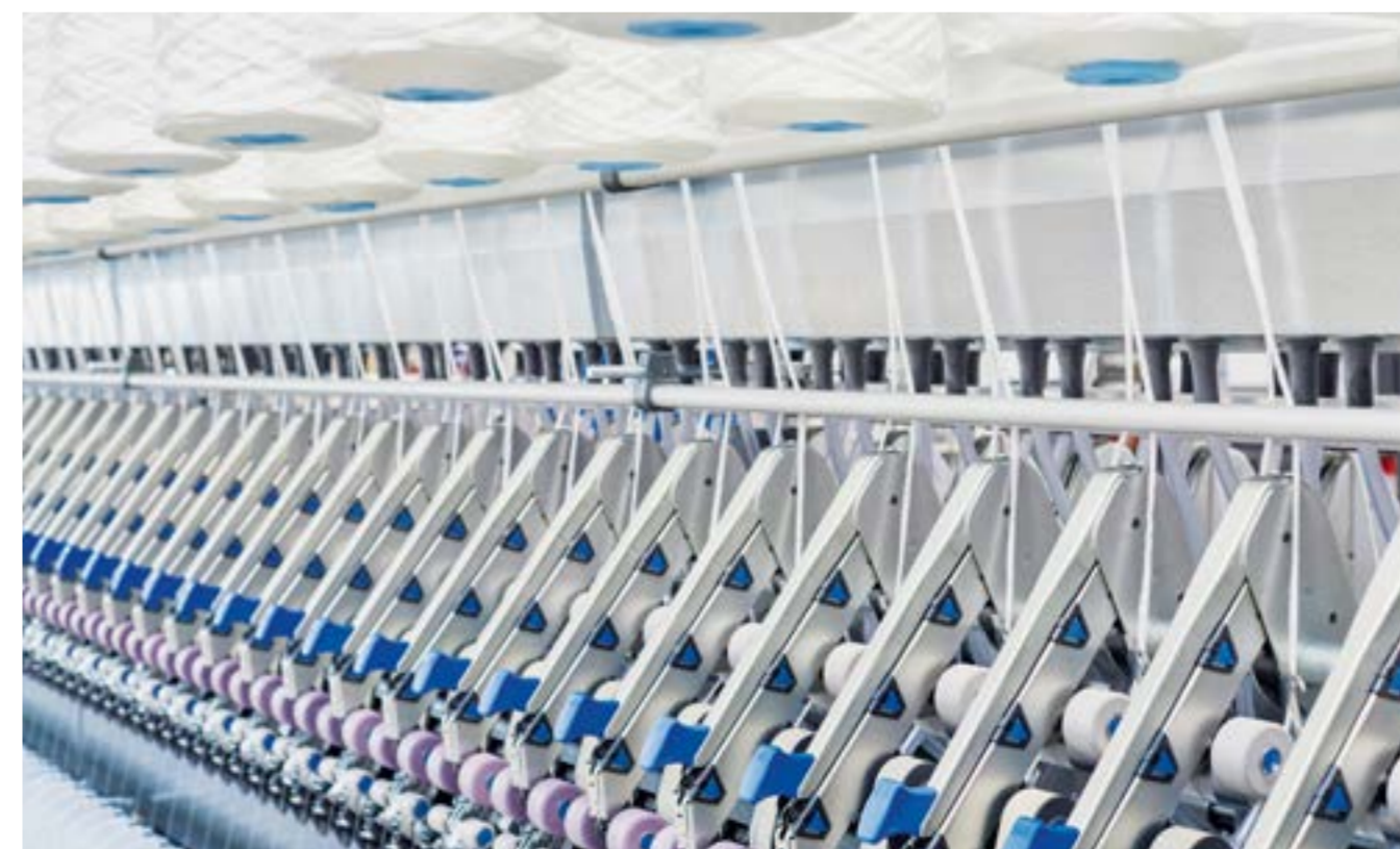
The ZI 451 worsted compact-spinning machine processes long staple fibres, such as wool.
