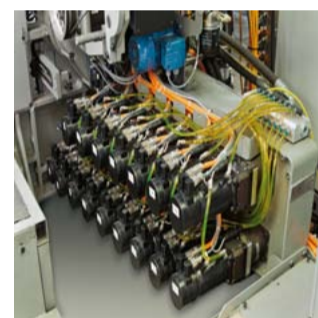
SF Smart Frames: electronic shedding by servomotor
