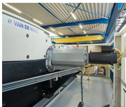
Servodrive Jacquard with electronic timing adjustment
