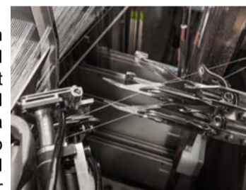
Redesigned weft inserton with improved rapier heads and weft cutng device
