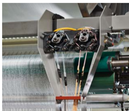
SE Smart Edges for servomotor sel-edge control
