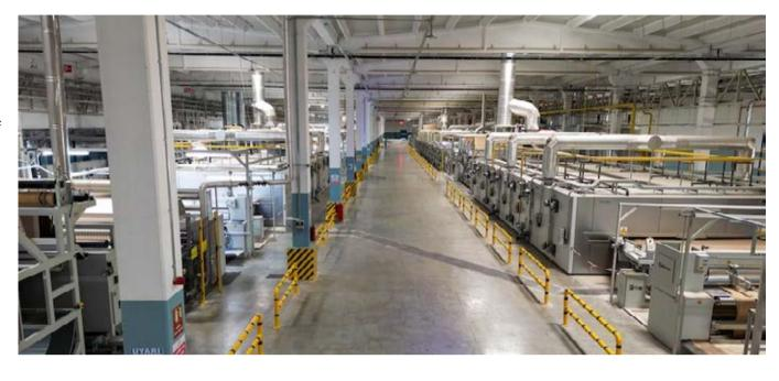
comforters or upholstery, as well as lightweight nonwovens for the hygiene industry such as ADL nonwovens, topsheets or backsheets can be finished on the air-through thermofusion ovens.
